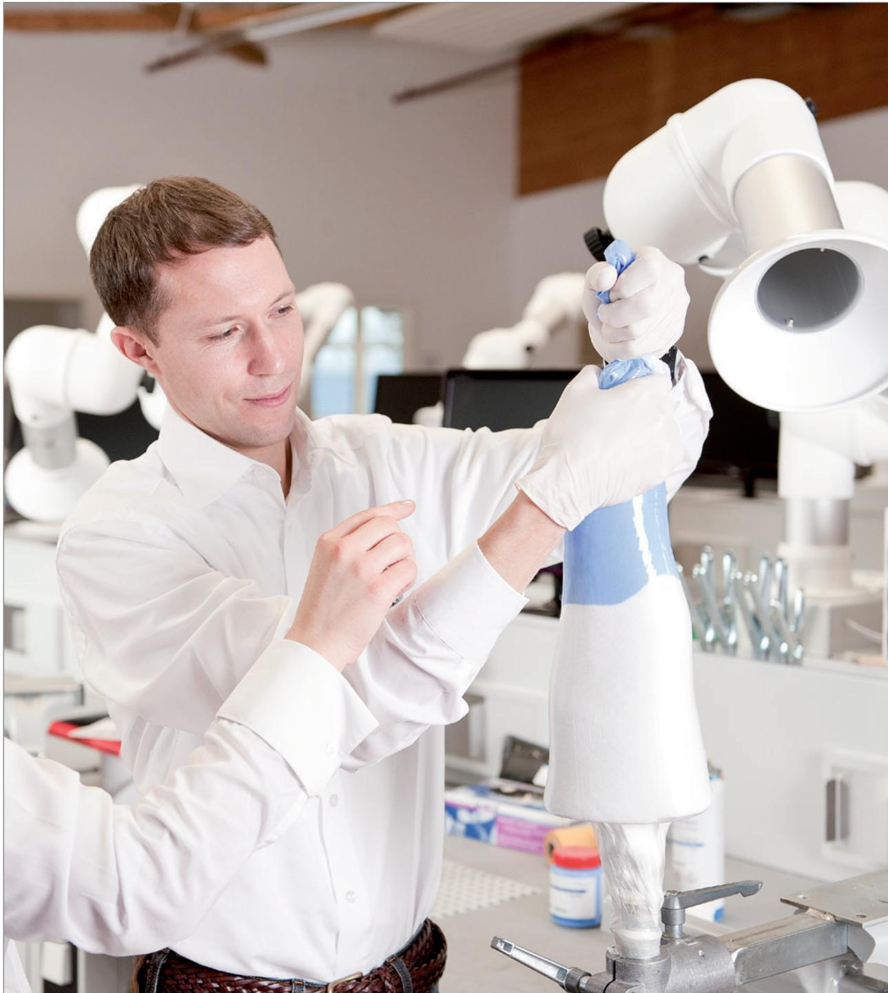
Due to their excellent wetting characteristics, acrylic- and epoxy-resins are especially suitable for laminating with carbon fiber materials. Epoxy-resin, however, is meanwhile more often used in orthopaedic technology, although it is a bit more demanding during processing than acrylic resin.
