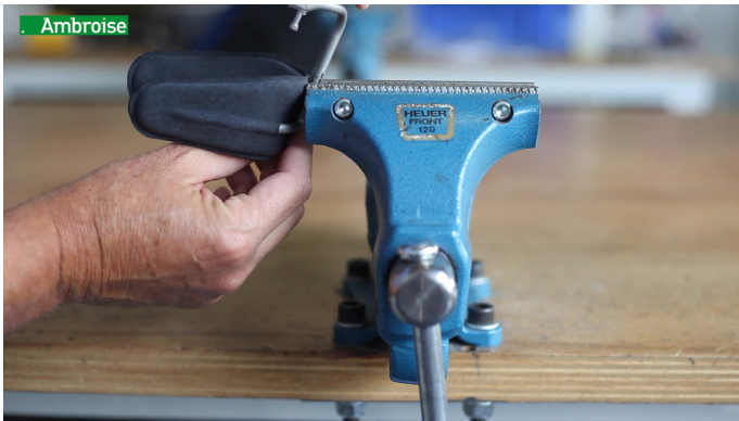
Step 5: Press the dot inwards with a vice in order to lock the hand support in place.
