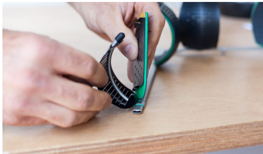
3. Remove the yellow strip, and press the flaps of the inner shell through the first groove of the outer shell.
