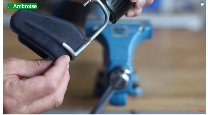
Step 6: The dot is now pressed into the tubes so the hand support is secured in place.
