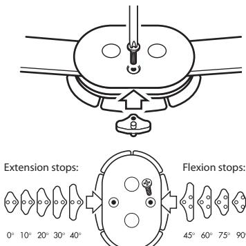
Both flexion and extension stops are supplied with the brace. The brace comes with a 10° extension stop already installed. The stops are labeled in degrees as follows;
