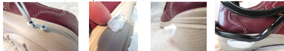
4 FORM JB WELD EPOXY OR SUGRU OVER SCREWS TO CREATE A LEDGE 3/8"-1/2"
