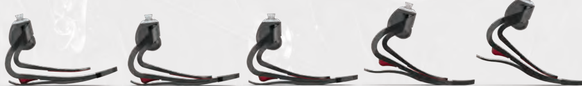
Ambulation while carrying additional load causes the heel plate to contact the stiffening bumper, followed by progressively greater contact between the primary and upper keels.
