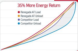
Products of equivalent size and stiffness category were tested according to an industry standard toe deflection test. Both products were loaded at 20 degrees to a 300 lb load.
